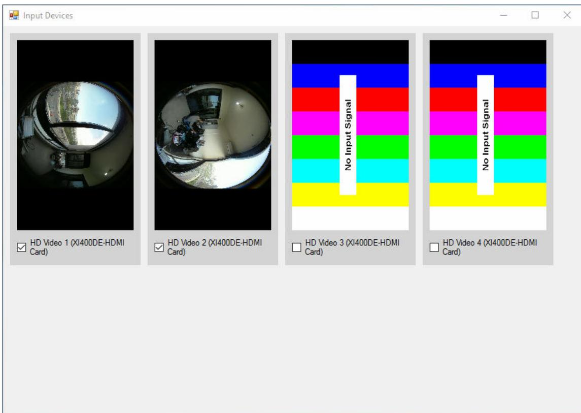
Press the “Select Input Devices” button and you will get a window that displays a preview for the connected cameras. Select which cameras you want to use and close the window. (Note that all the cameras will be unchecked by default).
