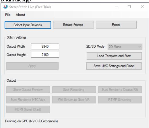
Run StereoStitch Live application, this step should always be done after the first step, and in case you restarted or connected a new camera, you should close and reopen the application again in order to detect new connected camera(s).
